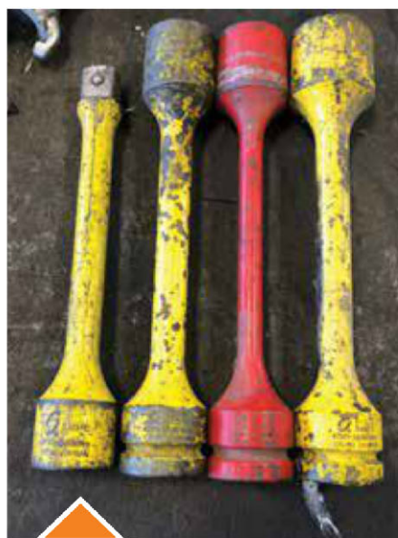
When using an air gun, the fastest way to maintain torque values is with torque sticks, which are typically calibrated to release in increments of 5 foot-pounds.
