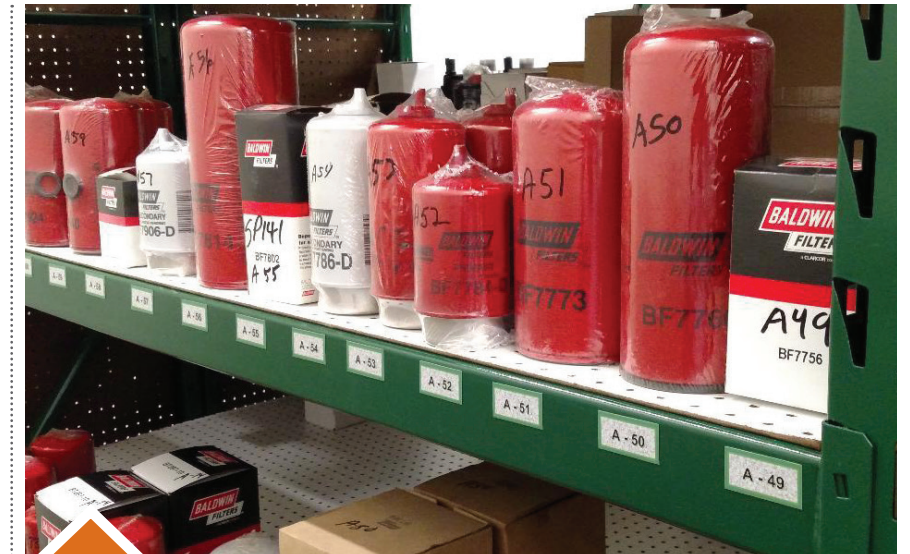
Keep filters and other contamination-sensitive supplies sealed until installation.
