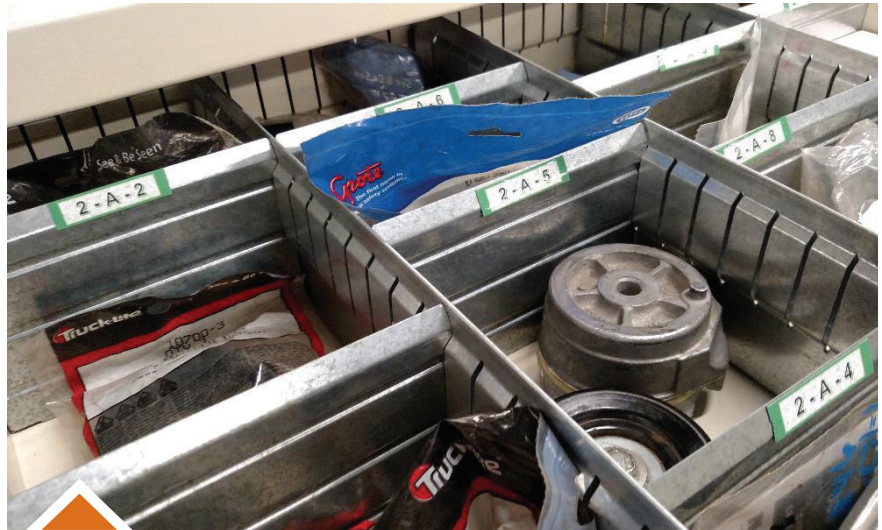
Compartmentalized drawer storage keeps parts from banging into each other and makes them easier to find.
