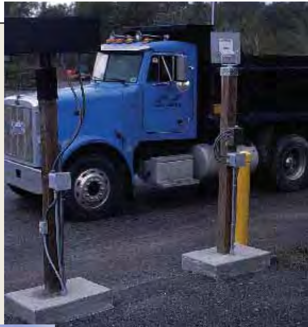
Above: When a trucker enters, an RF reader logs him in and a message board tells the trucker what scale and silo he needs to go to. Left: When the truck is loaded, the trucker picks up a ticket before heading out.
