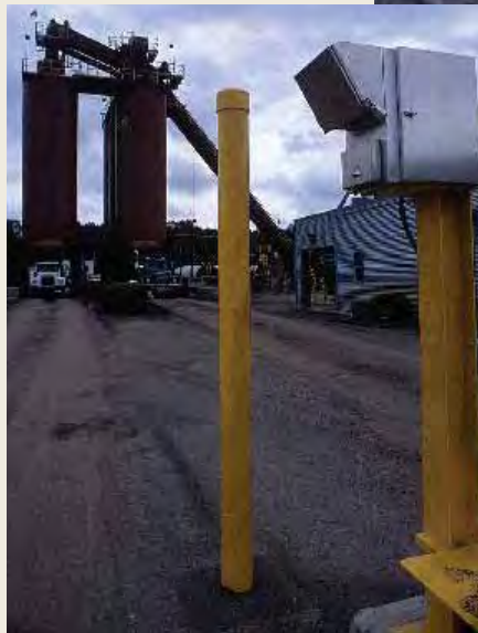
Above: When a trucker enters, an RF reader logs him in and a message board tells the trucker what scale and silo he needs to go to. Left: When the truck is loaded, the trucker picks up a ticket before heading out.
