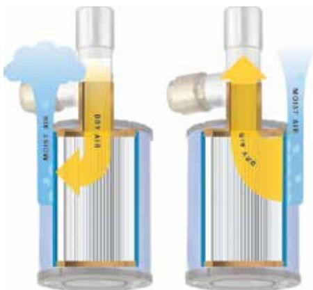
**▲▲▲** A desiccant breather on your bulk diesel storage tank can eliminate much of the water vapor that would otherwise condense on the inside of the tank when temperatures cool down overnight.
