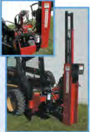
All models feature patented ultra-high molecular weight polyethylene slide blocks for maximum carriage contact surface to ensure optimum performance, minimum maintenance and long life. A level indicator is standard for easy, accurate alignment of the driver. Spring isolators dampen "whipping action" to extend spring life.
